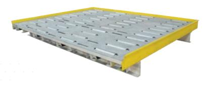
A heavy duty scale designed specifically for fast and accurate weighing of large containers. This allows loading and unloading in any direction, with steel tip-up container stops in key locations. A full steel deck plate allows safe walking over the scale for manually moving ULD's.
